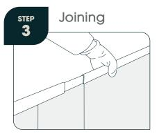
Where two pieces of edging meet, use joiners to connect the section securely.
