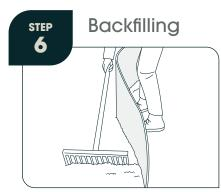
Once the edging is secure, use a rake or shovel to backfill the trench with the soil or material you initially removed.
