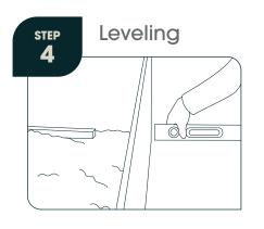
For straight sections use a builder's line set at the finished height of the edging. Check the top of the edging to ensure it is level and consistent along the entire length. Use a spirit level for curved sections.
